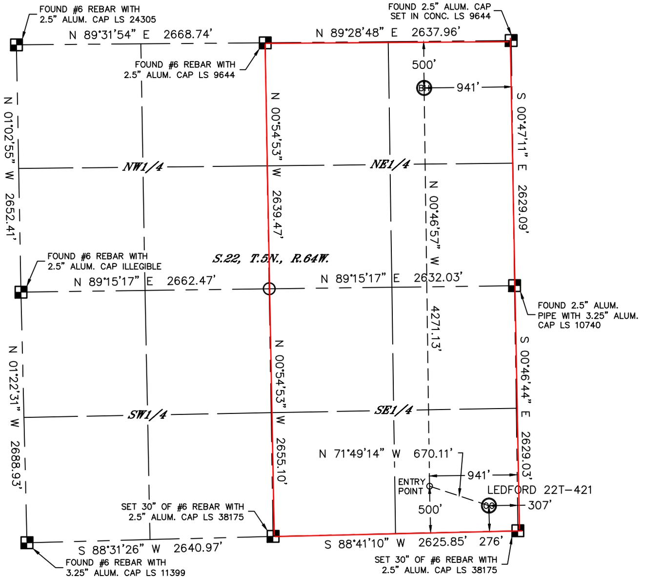
In accordance with a request from Jake Bragg with PDC ENERGY Lat40°, Inc. has determined the surface location of the LEDFORD 22T-421 to be 276' from the SOUTH line and 307' from the EAST line and the bottom hole to be 500' from the NORTH line and 941' from the EAST line as measured at right angles from the section lines of Section 22, Township 5 North, Range 64 West of the Sixth Principal Meridian, County of Weld, State of Colorado.
