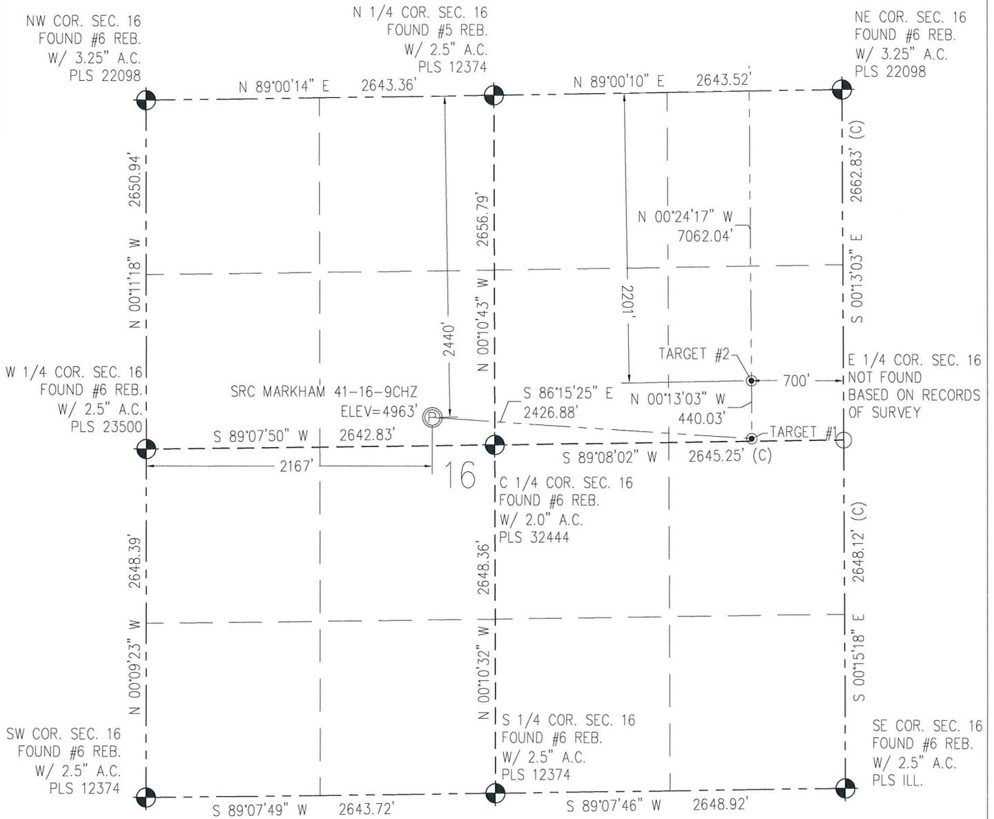
IN ACCORDANCE WITH A REQUEST FROM CRAIG RASMUSON - SYNERGY RESOURCES, BASELINE ENGINEERING CORP. HAS DETERMINED THE LOCATION OF THE SRC MARKHAM 41-16-9CHZ TO BE 2440' FNL AND 2167' FWL, AS MEASURED AT NINETY (90) DEGREES FROM THE SECTION LINE OF SECTION 16, TOWNSHIP 4 NORTH, RANGE 68 WEST AND THE BOTTOM HOLE LOCATION TO BE 460' FNL AND 700' FEL OF SECTION 9, TOWNSHIP 4 NORTH, RANGE 68 WEST, 6TH PRINCIPAL MERIDIAN, WELD COUNTY, COLORADO.
