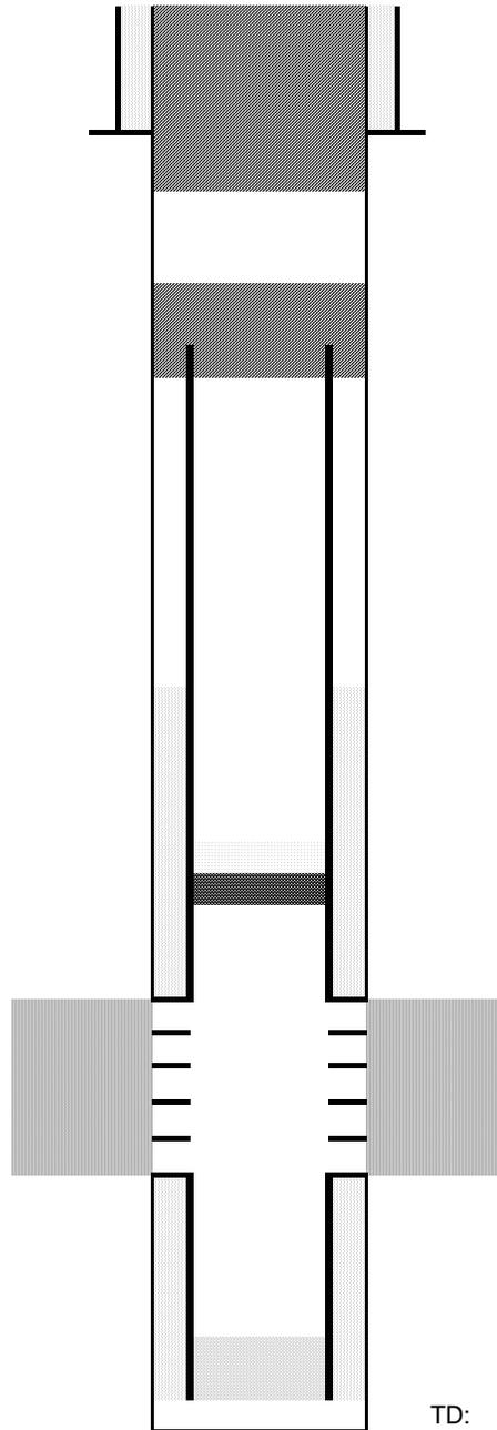
Cut surface casing off 6'-8' below surface.
