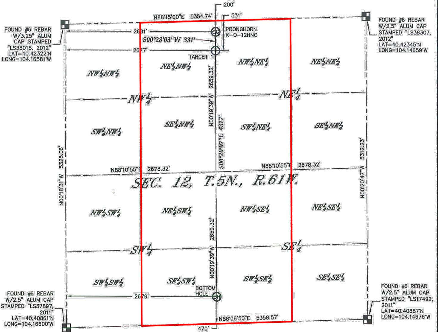
In accordance with a request from RANDY EDELEN with BONANZA CREEK ENERGY, INC., King Surveyors has determined the surface location of PRONGHORN K-O-12HNC to be 200' from the NORTH line and 2681' from the WEST line and the bottom
