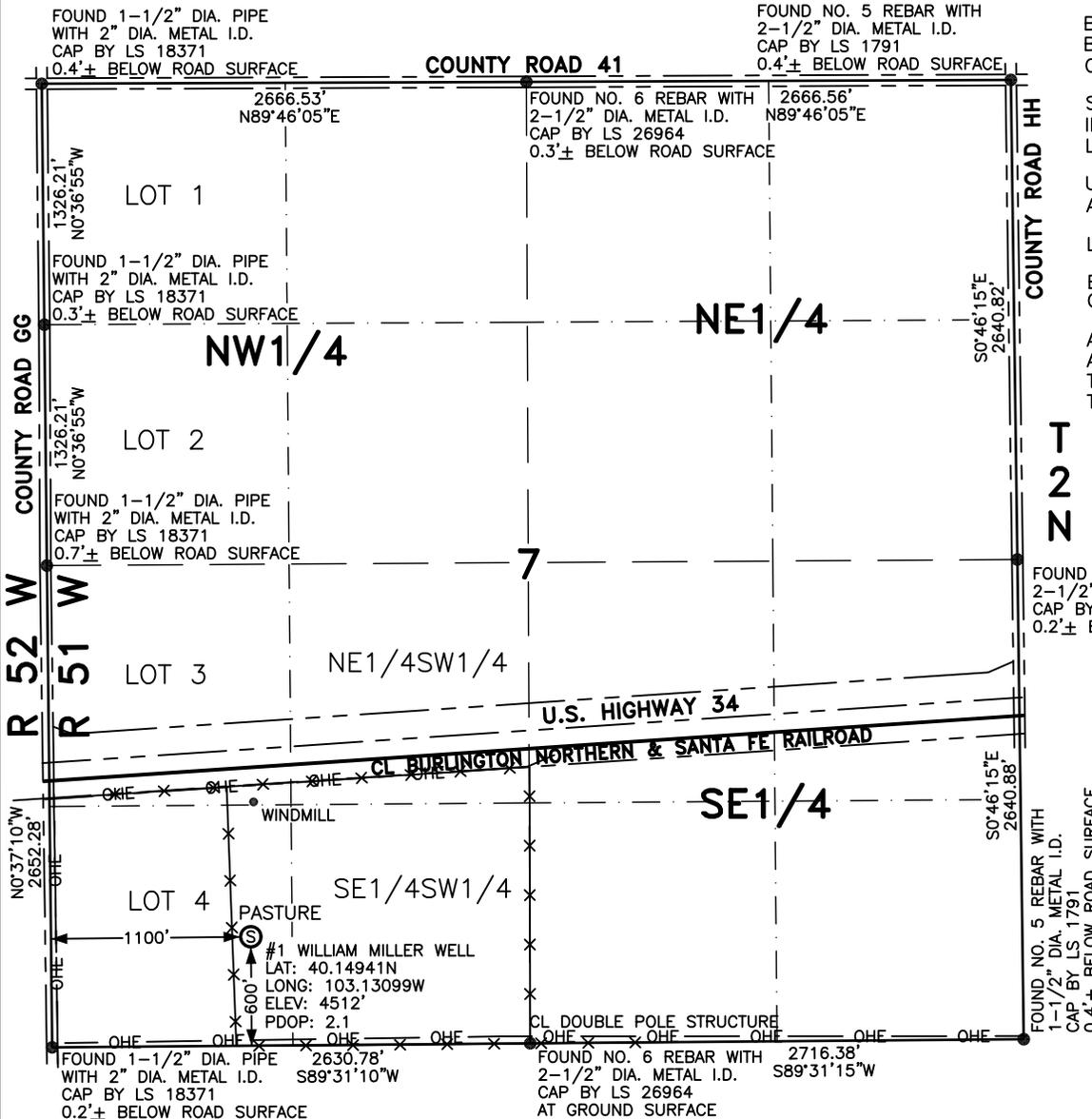
THIS WELL LOCATION PLAT HAS BEEN PREPARED FOR WINSLOW RESOURCES, INC. TO LOCATE THE #1 WILLIAM MILLER WELL BEING 1100 FEET FROM THE WEST LINE AND 600 FEET FROM THE SOUTH LINE IN THE SW1/4SW1/4 (LOT 4) OF SECTION 7, TOWNSHIP 2 NORTH, RANGE 51 WEST OF THE 6TH P.M., WASHINGTON COUNTY, COLORADO. THE SURFACE ELEVATION AT THIS POINT IS 4512 FEET. THIS IS NOT A LAND SURVEY PLAT.
