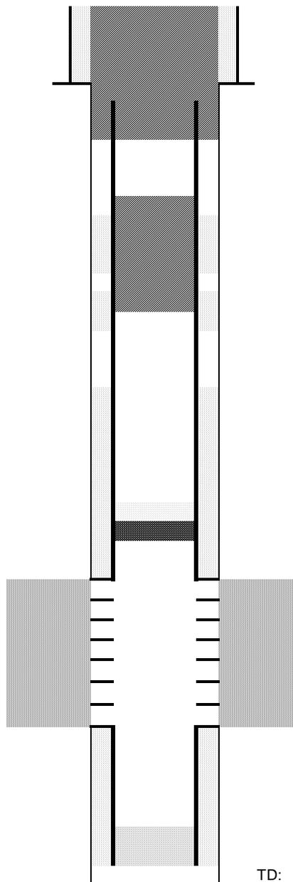
Cut surface casing off 6'-8' below surface.
