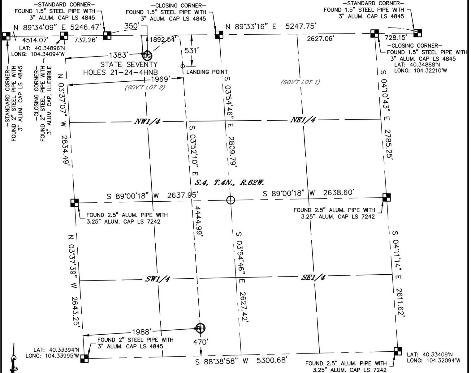
In accordance with a request from Keith Caplan with BONANZA CREEK ENERGY, INC. Lat40°, Inc. has determined the surface location of the STATE SEVENTY HOLES 21-24-4HNB to be 350' from the NORTH line and 1383' from the WEST line and the bottom hole to be 470' from the SOUTH line and 1988' from the WEST line as measured at right angles from the section lines of Section 4, Township 4 North, Range 62 West of the Sixth Principal Meridian, County of Weld, State of Colorado.
