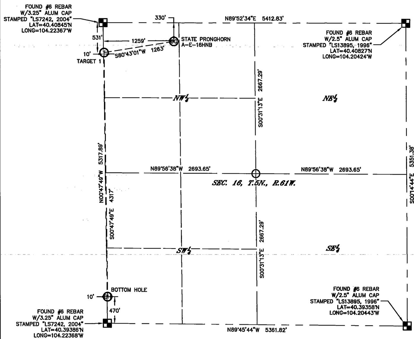
In accordance with a request from RANDY EDELEN with BONANZA CREEK ENERGY, INC. King Surveyors has determined the surface location of STATE PRONGHORN A-E-16HNB to be 330' from the NORTH line and 1259' from the WEST line and the bottom hole to be 470' from the SOUTH line and 10' from the WEST line, as measured at right angles, from the section lines of Section 16, Township 5 North, Range 61 West of the Sixth Principal Meridian, County of Weld, State of Colorado.
