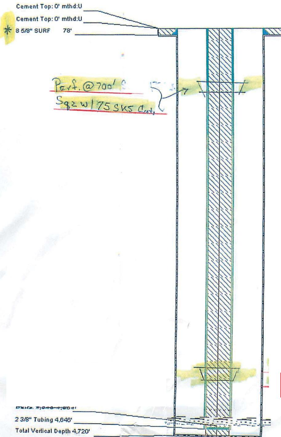
\* Drilling contract called for setting 500' of surface pipe. Contractor set 78'. Therefore, Otis Sliding Sleeve was set to 640 feet K.B., set 16 joints below bottom of surface pipe. Spotted 1,000 gallons E.T.S. chem. gel through Otis Sleeve and circulated to surface.
