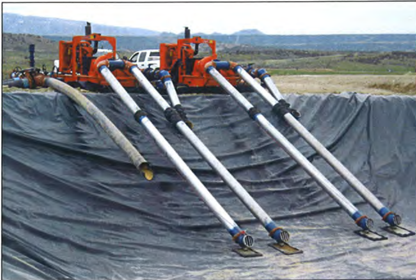
Photo 2. Example of water pumps with stinger pipes reaching down into a pit.
