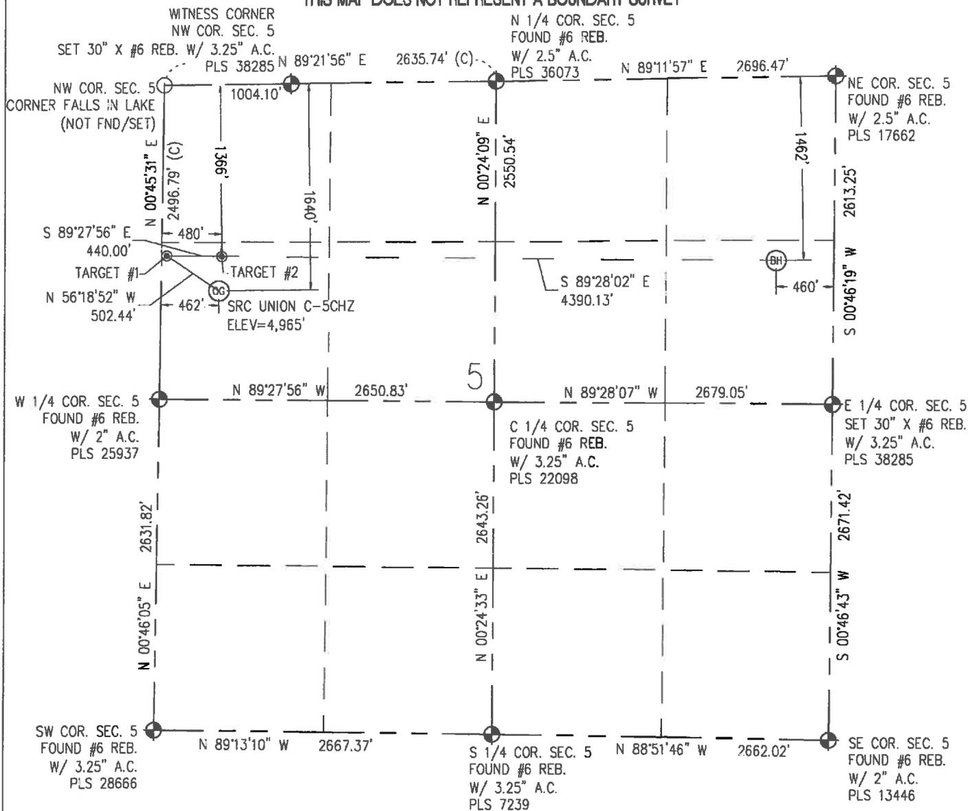
IN ACCORDANCE WITH A REQUEST FROM CRAIG RASMUSON - SYNERGY RESOURCES, BASELINE ENGINEERING CORP. HAS DETERMINED THE LOCATION OF THE SRC UNION C-5CHZ TO BE 1640' FNL AND 462' FWL, AS MEASURED AT NINETY (90) DEGREES FROM THE SECTION LINE OF SECTION 5, TOWNSHIP 2 NORTH, RANGE 68 WEST AND THE BOTTOM HOLE LOCATION TO BE 1462' FNL AND 460' FEL OF SECTION 5, TOWNSHIP 2 NORTH, RANGE 68 WEST, 6TH PRINCIPAL MERIDIAN, WELD COUNTY, COLORADO.
