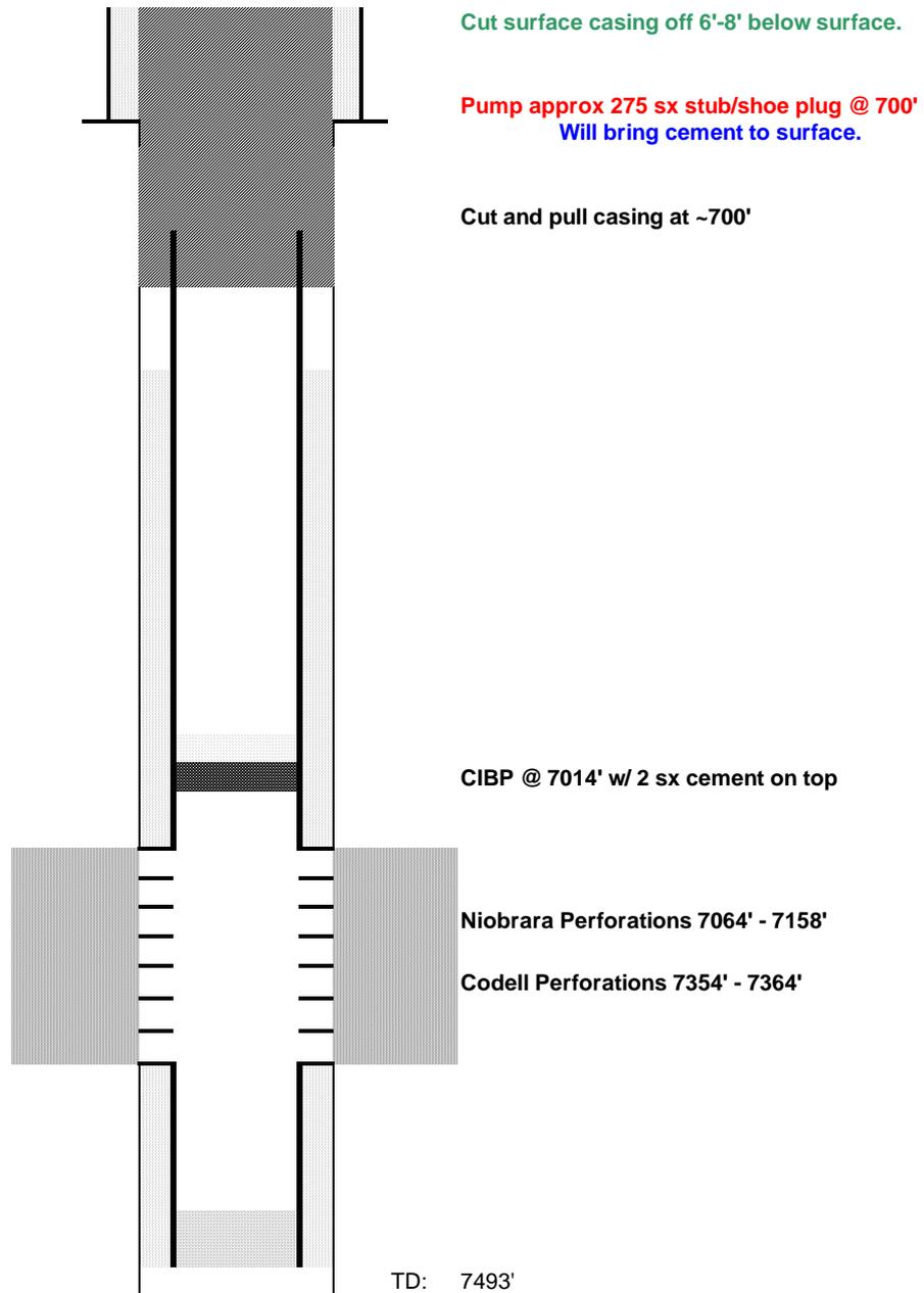
Cut surface casing off 6'-8' below surface.
