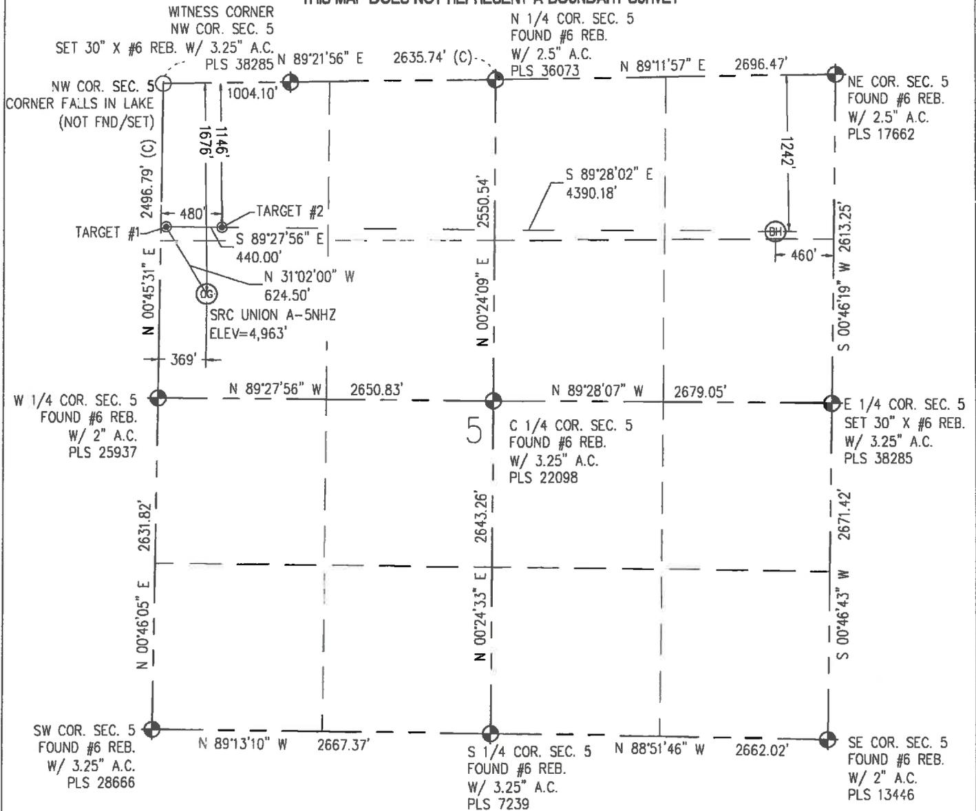
IN ACCORDANCE WITH A REQUEST FROM CRAIG RASMUSON - SYNERGY RESOURCES, BASELINE ENGINEERING CORP. HAS DETERMINED THE LOCATION OF THE SRC UNION A-5NHZ TO BE 1676' FNL AND 369' FWL, AS MEASURED AT NINETY (90) DEGREES FROM THE SECTION LINE OF SECTION 5, TOWNSHIP 2 NORTH, RANGE 68 WEST AND THE BOTTOM HOLE LOCATION TO BE 1242' FNL AND 460' FEL OF SECTION 5, TOWNSHIP 2 NORTH, RANGE 68 WEST, 6TH PRINCIPAL MERIDIAN, WELD COUNTY, COLORADO.
