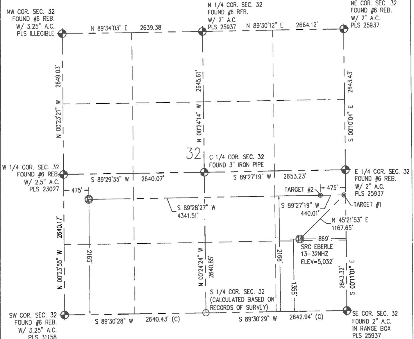
IN ACCORDANCE WITH A REQUEST FROM CRAIG RASMUSON - SYNERGY RESOURCES, BASELINE ENGINEERING CORP. HAS DETERMINED THE LOCATION OF THE SRC EBERLE 13-32NHZ TO BE 1355' FSL AND 869' FEL, AS MEASURED AT NINETY (90) DEGREES FROM THE SECTION LINE OF SECTION 32, TOWNSHIP 1 NORTH, RANGE 66 WEST AND THE BOTTOM HOLE LOCATION TO BE 2165' FSL AND 475' FWL OF SECTION 32, TOWNSHIP 1 NORTH, RANGE 66 WEST, 6TH PRINCIPAL MERIDIAN, WELD COUNTY, COLORADO.
