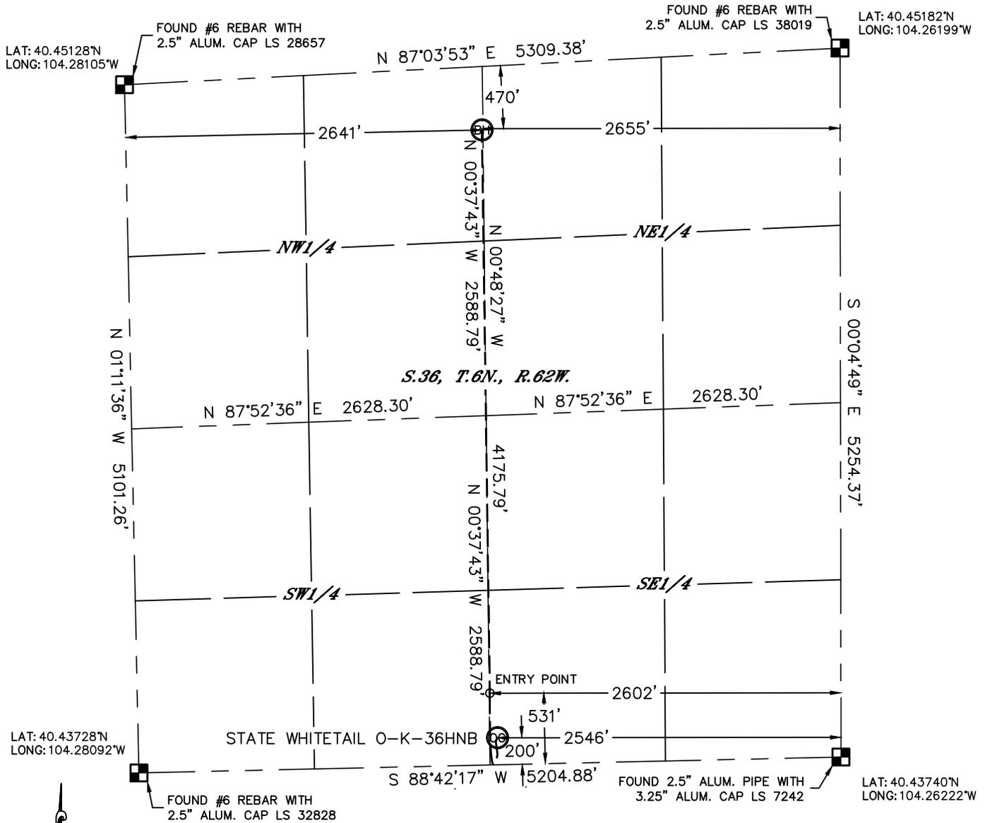
In accordance with a request from Keith Caplan with BONANZA CREEK ENERGY, INC. Lat40°, Inc. has determined the surface location of the STATE WHITETAIL O-K-36HNB to be 200' from the SOUTH line and 2546' from the EAST line and the bottom hole to be 470' from the NORTH line and 2655' from the EAST line as measured at right angles from the section lines of Section 36, Township 6 North, Range 62 West of the Sixth Principal Meridian, County of Weld, State of Colorado.
