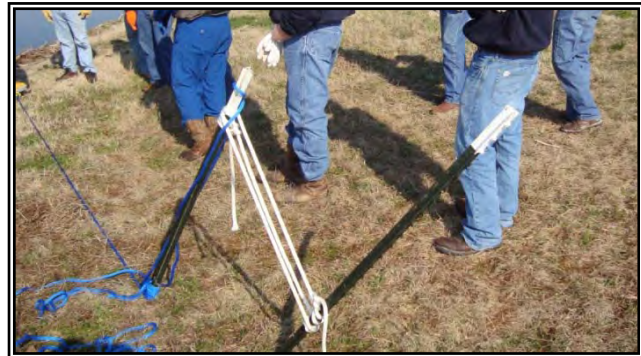
Anchoring Boom on Land
