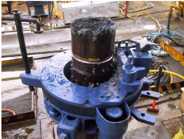
Figure F.6 – Lathe Cutter in Use on 5" Drill Pipe
