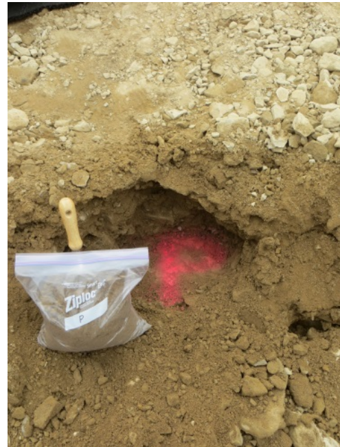
Photo 8 – Confirmation sampling at excavation perimeter
