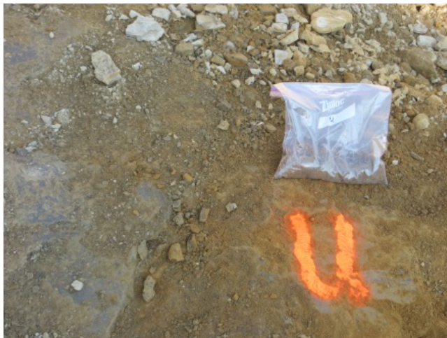
Photo 9 – Confirmation sampling of bedrock on excavation floor
