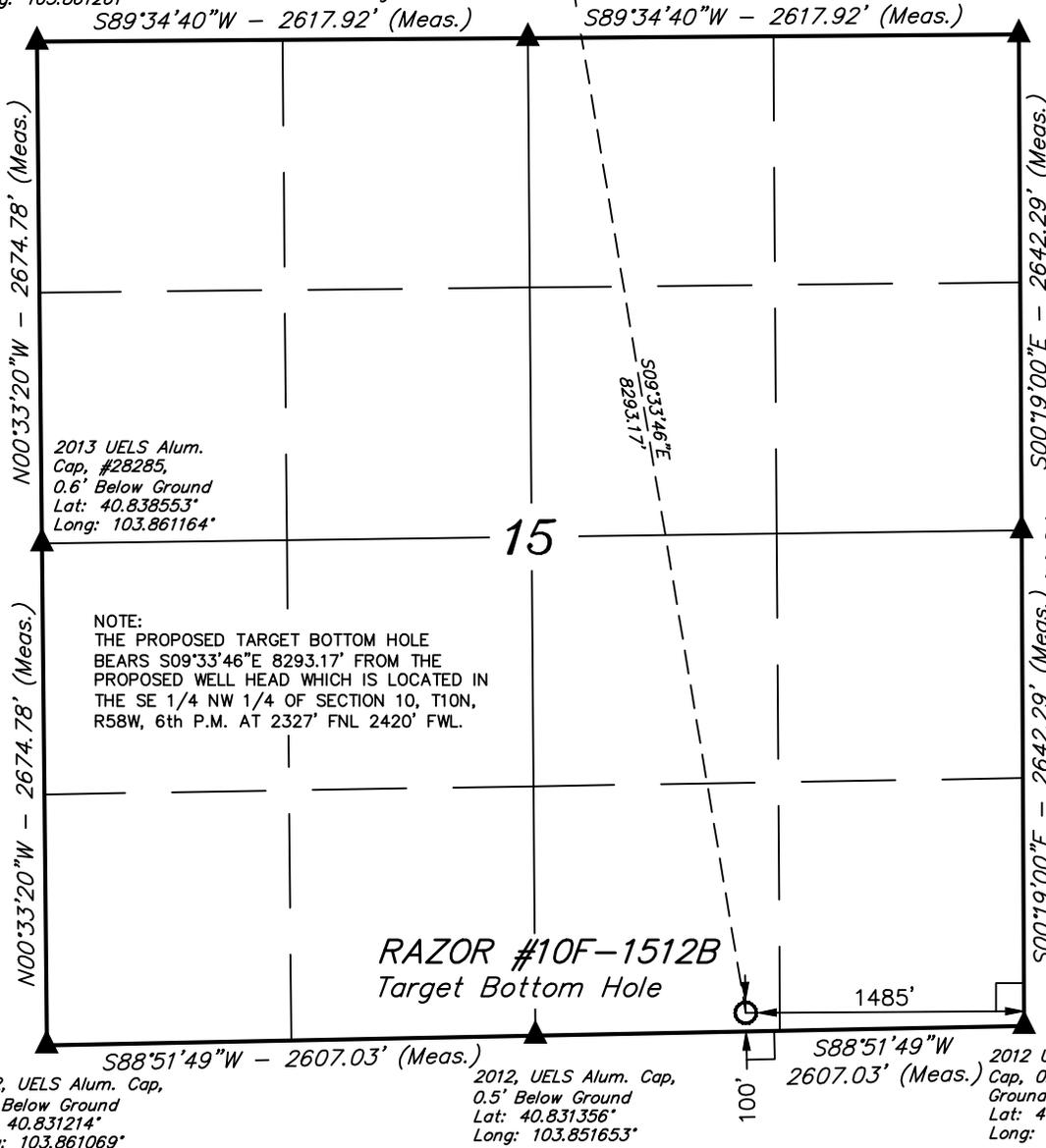
Well location, RAZOR #10F-1512B (TARGET BOTTOM HOLE), located as shown in the SW 1/4 SE 1/4 of Section 15, T10N, R58W, 6th P.M., Weld County, Colorado.
