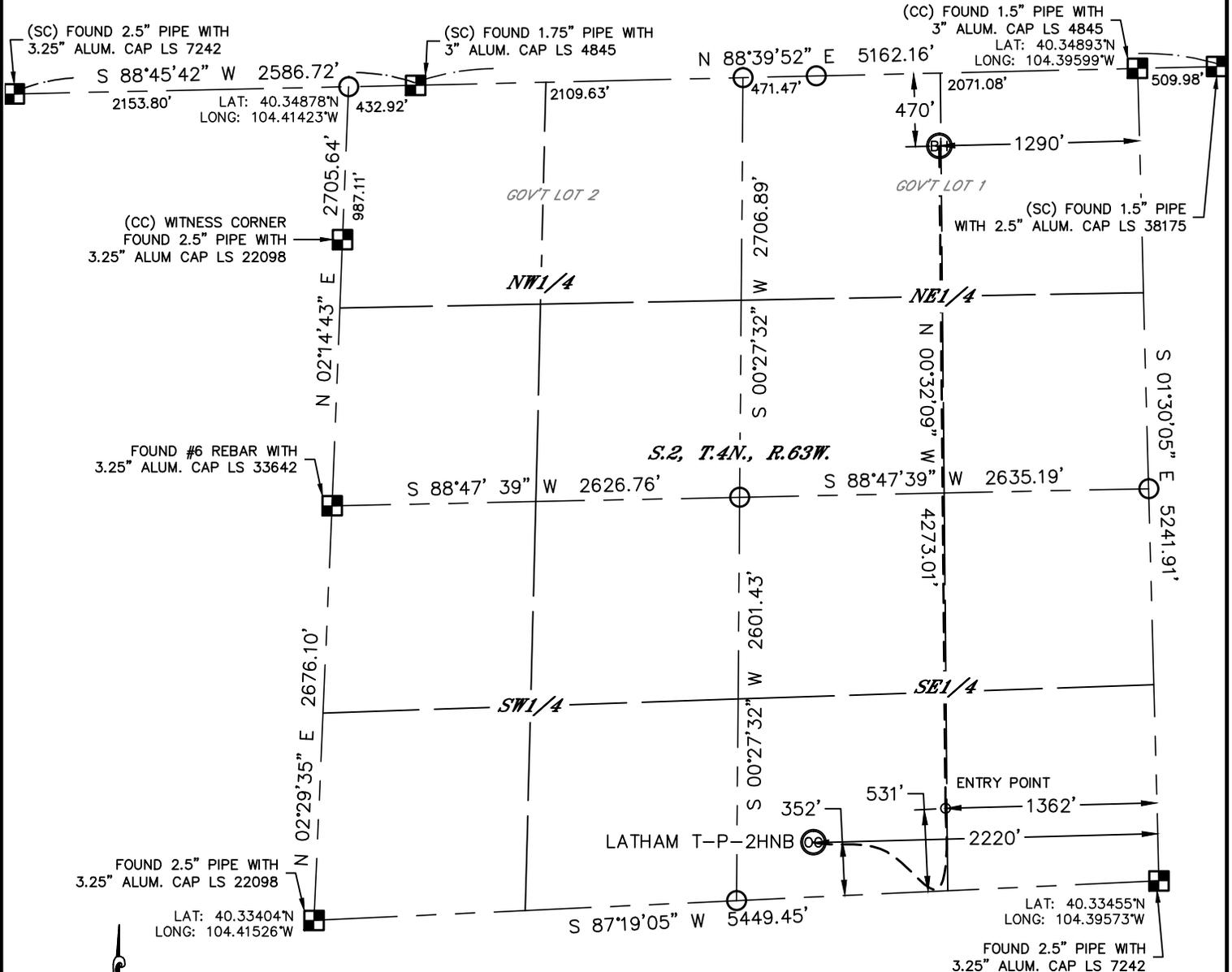
In accordance with a request from Keith Caplan with BONANZA CREEK ENERGY, INC. Lat40°, Inc. has determined the surface location of the LATHAM T-P-2HNB to be 352' from the SOUTH line and 2220' from the EAST line and the bottom hole to be 470' from the NORTH line and 1290' from the EAST line as measured at right angles from the section lines of Section 2, Township 4 North, Range 63 West of the Sixth Principal Meridian, County of Weld, State of Colorado.
