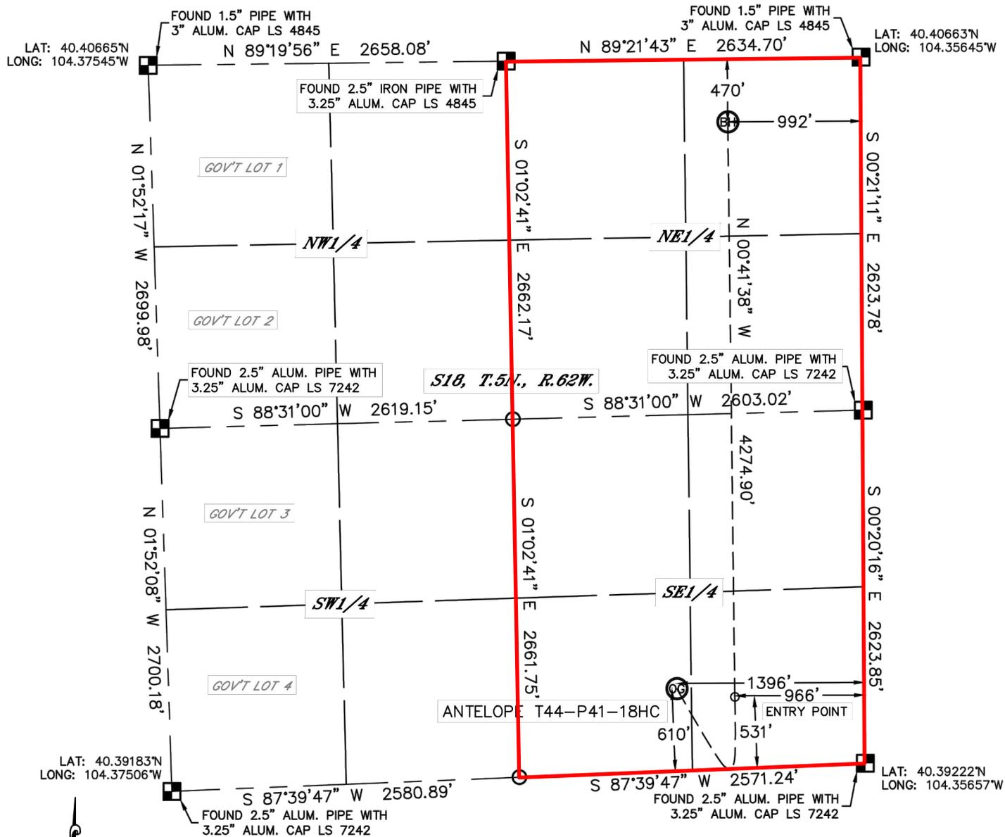
In accordance with a request from Keith Caplan with BONANZA CREEK ENERGY, INC. Lat40°, Inc. has determined the surface location of the ANTELOPE T44-P41-18HC to be 610' from the SOUTH line and 1396' from the EAST line and the bottom hole to be 470' from the NORTH line and 992'
