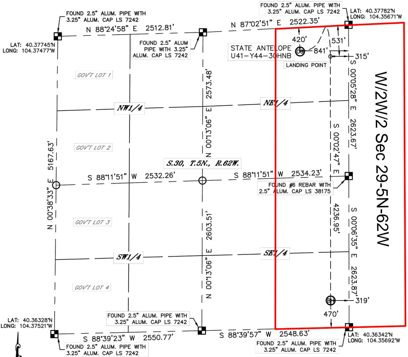
In accordance with a request from Keith Caplan with BONANZA CREEK ENERGY, INC. Lat40°, Inc. has determined the surface location of the STATE ANTELOPE U41-Y44-30HNB to be 420' from the NORTH line and 841' from the EAST line and the bottom hole to be 470' from the SOUTH line and 319' from the EAST line as measured at right angles from the section lines of Section 30, Township 5
