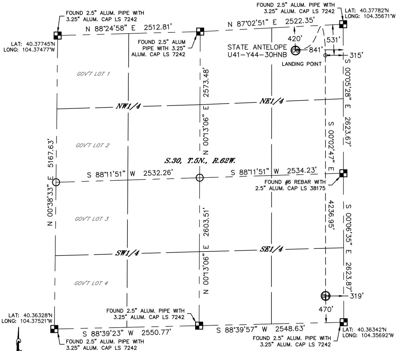
In accordance with a request from Keith Caplan with BONANZA CREEK ENERGY, INC. Lat40°, Inc. has determined the surface location of the STATE ANTELOPE U41-Y44-30HNB to be 420' from the NORTH line and 841' from the EAST line and the bottom hole to be 470' from the SOUTH line and 319' from the EAST line as measured at right angles from the section lines of Section 30, Township 5 North, Range 62 West of the Sixth Principal Meridian, County of Weld, State of Colorado.
