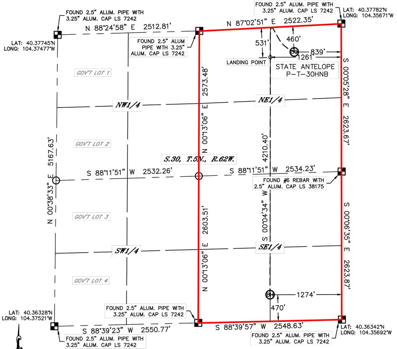
In accordance with a request from Keith Caplan with BONANZA CREEK ENERGY, INC., Lat40°, Inc. has determined the surface location of the STATE ANTELOPE P-T-30HNB to be 460' from the NORTH line and 839' from the EAST line and the bottom hole to be 470' from the SOUTH line and 1274'
