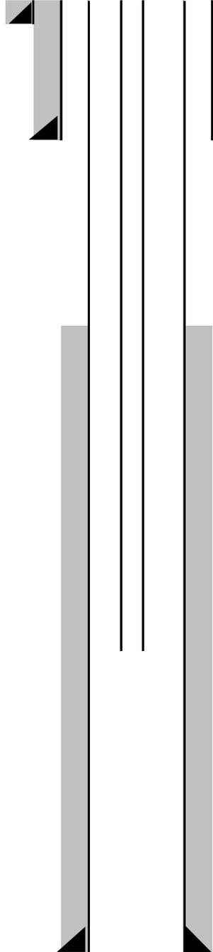
Conductor 26" Hole 18" casing/liner 40' W/ 15 Sks cmt
