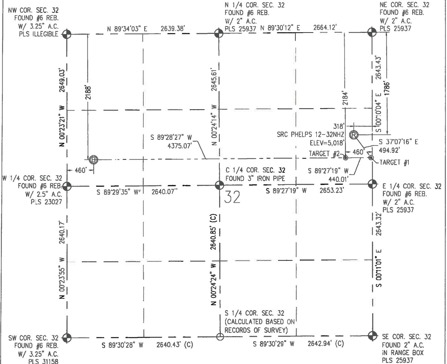
IN ACCORDANCE WITH A REQUEST FROM CRAIG RASMUSON - SYNERGY RESOURCES, BASELINE ENGINEERING CORP. HAS DETERMINED THE LOCATION OF THE SRC PHELPS 12-32NHZ AND 318' FEL, AS MEASURED AT NINETY (90) DEGREES FROM THE SECTION LINE OF SECTION 32, TOWNSHIP 1 NORTH, RANGE 66 WEST AND THE BOTTOM HOLE LOCATION TO BE 2'88' FNL AND 460' FWL OF SECTION 32, TOWNSHIP 1 NORTH, RANGE 66 WEST, 6TH PRINCIPAL MERIDIAN, WELD COUNTY, COLORADO.
