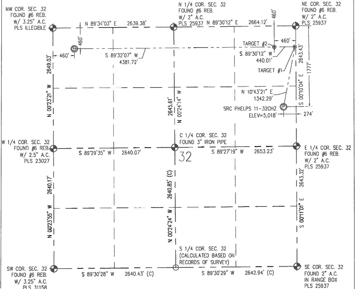
IN ACCORDANCE WITH A REQUEST FROM CRAIG RASMUSON - SYNERGY RESOURCES, BASELINE ENGINEERING CORP. HAS DETERMINED THE LOCATION OF THE SRC PHELPS 11-32CHZ TO BE 1,777' FNL AND 274' FEL, AS MEASURED AT NINETY (90) DEGREES FROM THE SECTION LINE OF SECTION 32, TOWNSHIP 1 NORTH, RANGE 66 WEST AND THE BOTTOM HOLE LOCATION TO BE 460' FNL AND 460' FWL OF SECTION 32, TOWNSHIP 1 NORTH, RANGE 66 WEST, 6TH PRINCIPAL MERIDIAN, WELD COUNTY, COLORADO.
