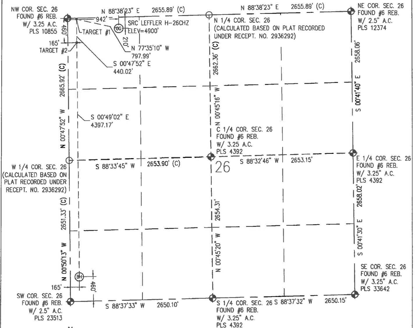
IN ACCORDANCE WITH A REQUEST FROM CRAIG RASMUSON - SYNERGY RESOURCES, BASELINE ENGINEERING CORP. HAS DETERMINED THE LOCATION OF THE SRC LEFFLER H-26CHZ TO BE 210' FNL AND 942' FWL, AS MEASURED AT NINETY (90) DEGREES FROM THE SECTION LINE OF SECTION 26, TOWNSHIP 7 NORTH, RANGE 66 WEST AND THE BOTTOM HOLE LOCATION TO BE 460' FSL AND 165' FWL OF SECTION 26, TOWNSHIP 7 NORTH, RANGE 66 WEST, 6TH PRINCIPAL MERIDIAN, WELD COUNTY, COLORADO.
