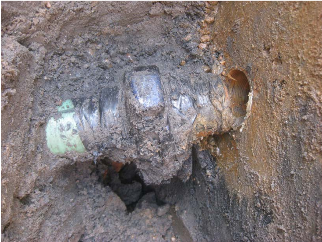
The dump line nipple failed where it was attached to the concrete pit
