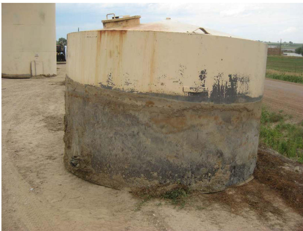
Steel water pit after removal. No indication of failure was observed.
