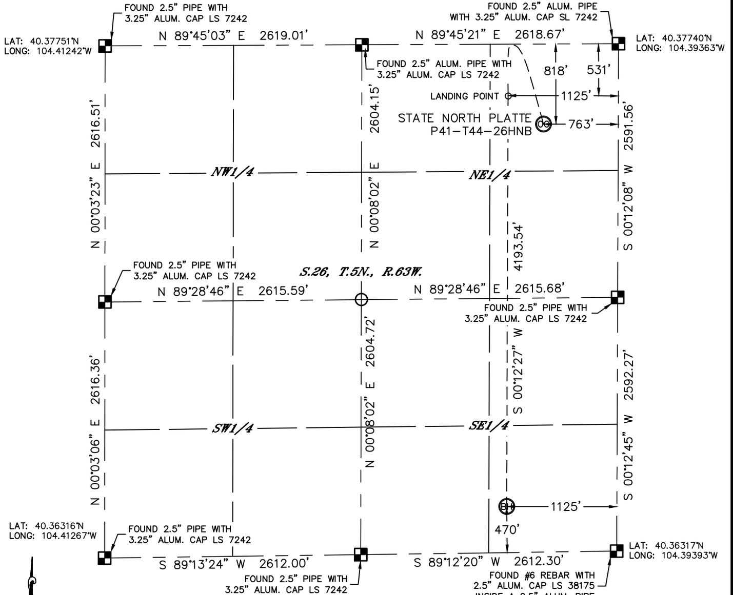
In accordance with a request from Michael Meagher with BONANZA CREEK ENERGY, INC. Lat40°, Inc. has determined the surface location of the STATE NORTH PLATTE P41-T44-26HNB to be 818' from the NORTH line and 763' from the EAST line and the bottom hole to be 470' from the SOUTH line and 1125' from the EAST line as measured at right angles from the section lines of Section 26, Township 5 North, Range 63 West of the Sixth Principal Meridian, County of Weld, State of Colorado.
