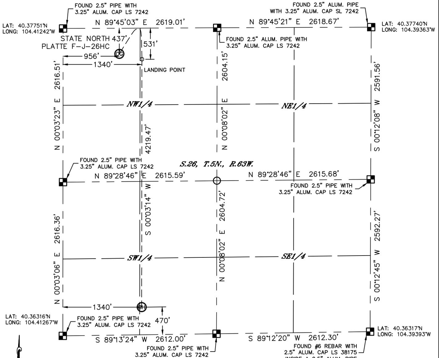
In accordance with a request from Michael Meagher with BONANZA CREEK ENERGY, INC. Lat40°, Inc. has determined the surface location of the STATE NORTH PLATTE F-J-26HC to be 437' from the NORTH line and 956' from the WEST line and the bottom hole to be 470' from the SOUTH line and 1340' from the WEST line as measured at right angles from the section lines of Section 26, Township 5 North, Range 63 West of the Sixth Principal Meridian, County of Weld, State of Colorado.
