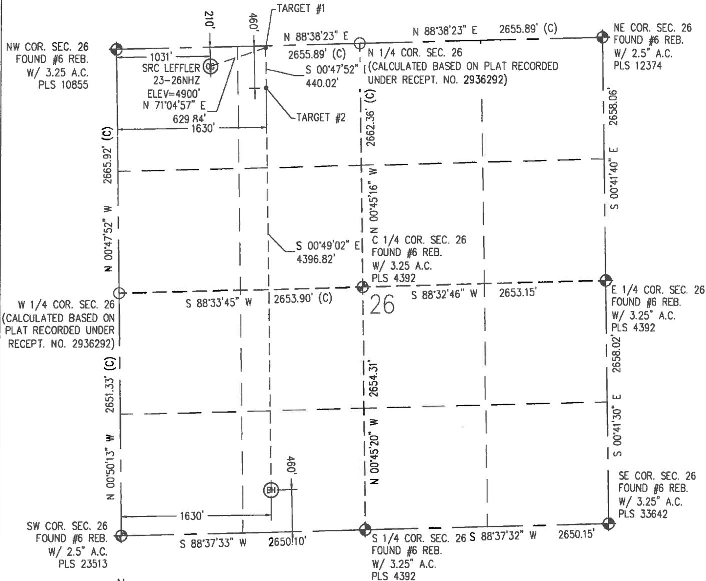
IN ACCORDANCE WITH A REQUEST FROM CRAIG RASMUSON - SYNERGY RESOURCES, BASELINE ENGINEERING CORP. HAS DETERMINED THE LOCATION OF THE SRC LEFFLER 23-26NHZ TO BE 210' FNL AND 1031' FWL, AS MEASURED AT NINETY (90) DEGREES FROM THE SECTION LINE OF SECTION 26, TOWNSHIP 7 NORTH, RANGE 66 WEST AND THE BOTTOM HOLE LOCATION TO BE 460' FSL AND 1630' FWL OF SECTION 26, TOWNSHIP 7 NORTH, RANGE 66 WEST, 6TH PRINCIPAL MERIDIAN, WELD COUNTY, COLORADO.
