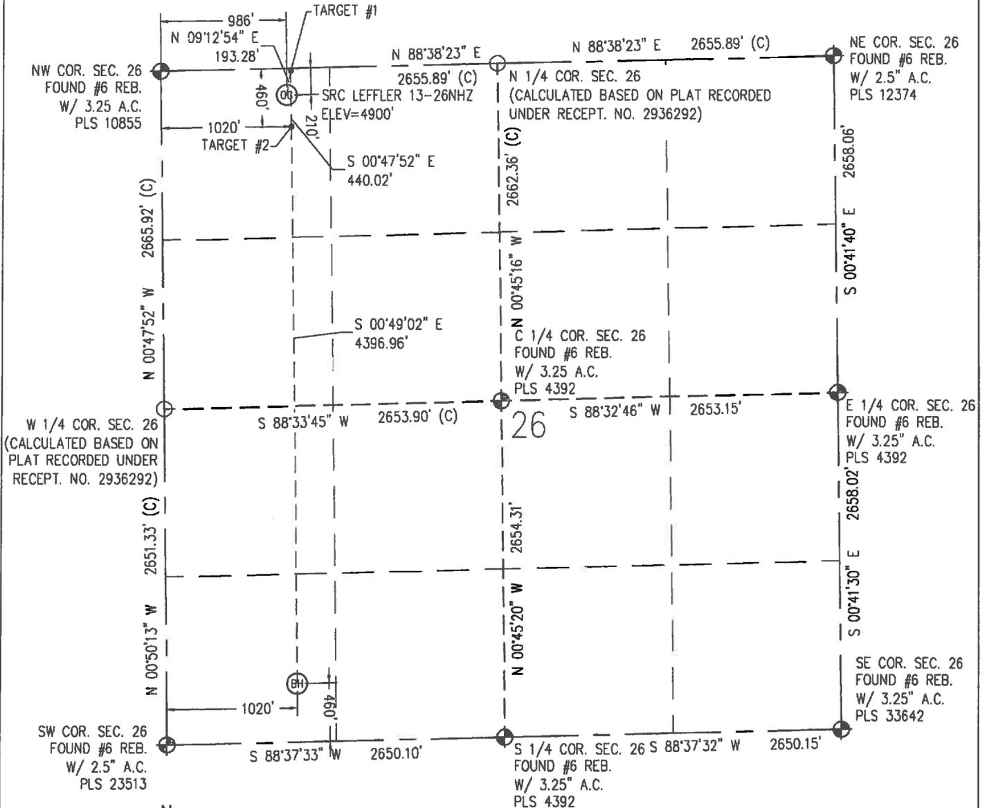
IN ACCORDANCE WITH A REQUEST FROM CRAIG RASMUSON - SYNERGY RESOURCES, BASELINE ENGINEERING CORP. HAS DETERMINED THE LOCATION OF THE SRC LEFFLER 13-26NHZ TO BE 210' FNL AND 986' FWL, AS MEASURED AT NINETY (90) DEGREES FROM THE SECTION LINE OF SECTION 26, TOWNSHIP 7 NORTH, RANGE 66 WEST AND THE BOTTOM HOLE LOCATION TO BE 460' FSL AND 1020' FWL OF SECTION 26, TOWNSHIP 7 NORTH, RANGE 66 WEST, 6TH PRINCIPAL MERIDIAN, WELD COUNTY, COLORADO.
