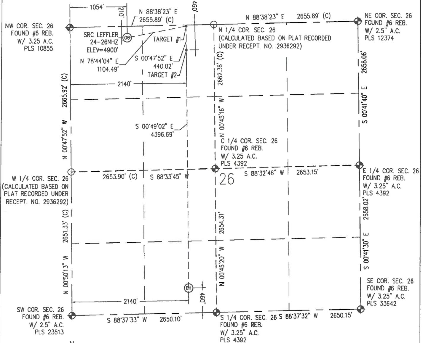
IN ACCORDANCE WITH A REQUEST FROM CRAIG RASMUSON - SYNERGY RESOURCES, BASELINE ENGINEERING CORP. HAS DETERMINED THE LOCATION OF THE SRC LEFFLER 24-26NHZ TO BE 210' FNL AND 1054' FWL, AS MEASURED AT NINETY (90) DEGREES FROM THE SECTION LINE OF SECTION 26, TOWNSHIP 7 NORTH, RANGE 66 WEST AND THE BOTTOM HOLE LOCATION TO BE 460' FSL AND 2140' FWL OF SECTION 26, TOWNSHIP 7 NORTH, RANGE 66 WEST, 6TH PRINCIPAL MERIDIAN, WELD COUNTY, COLORADO.
