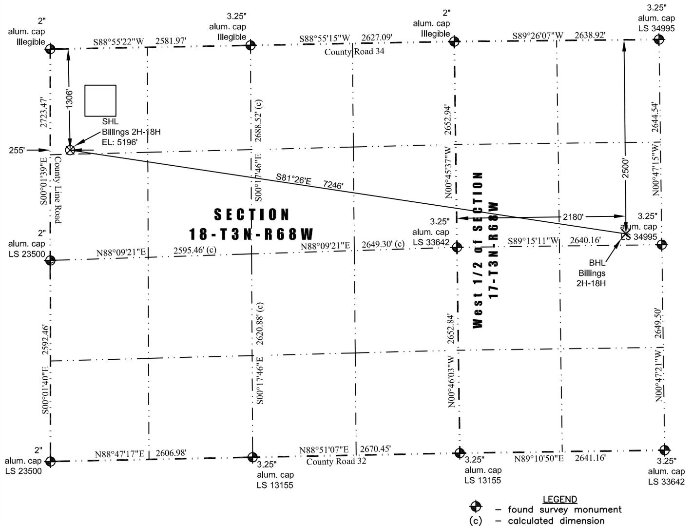
In accordance with a request from Jay Knutson of EnCana Oil & Gas (USA) Inc., JR Land Surveying, LLC has determined the location of the **Billings 2H-18H** well site to be SHL: 1306' FNL and 255' FWL, (BHL: 2500' FNL and 2180' FWL) as measured at ninety (90) degrees from the section lines of Section 18 and Section 17, Township 3 North, Range 68 West, 6th Principal Meridian, County of Weld, CO.
