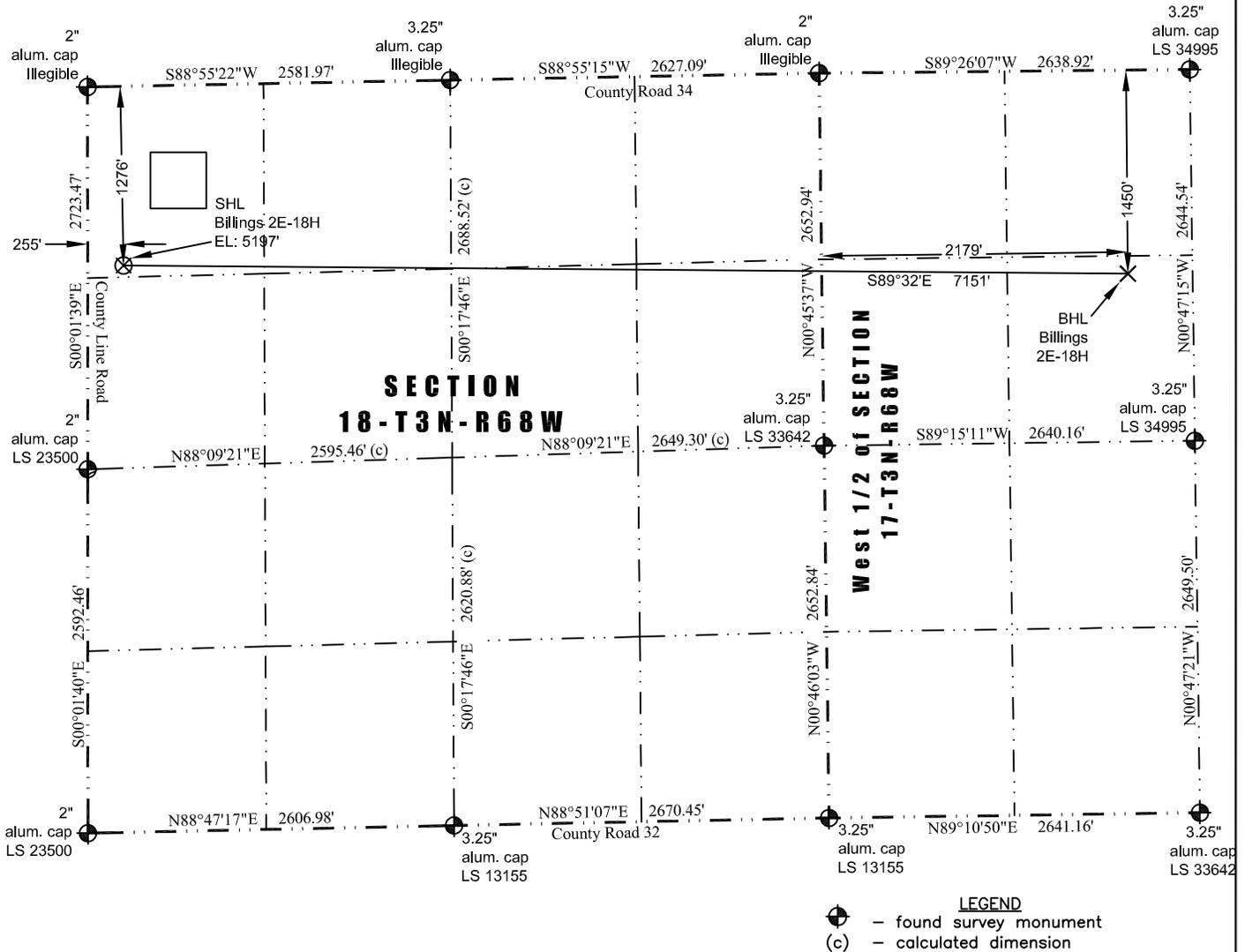
In accordance with a request from Jay Knutson of EnCana Oil & Gas (USA) Inc., JR Land Surveying, LLC has determined the location of the **Billings 2E-18H** well site to be SHL: 1276' FNL and 255' FWL, (BHL: 1450' FNL and 2179' FWL) as measured at ninety (90) degrees from the section lines of Section 18 and Section 17, Township 3 North, Range 68 West, 6th Principal Meridian, County of Weld, CO.
