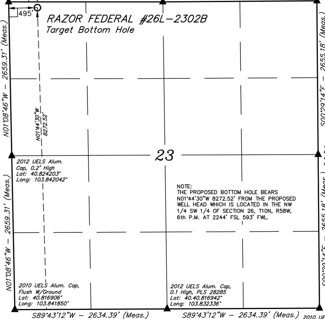
Well location, RAZOR FEDERAL #26L-2302B (TARGET BOTTOM HOLE), located as shown in the NW 1/4 NW 1/4 of Section 23, T10N, R58W, 6th P.M., Weld County, Colorado.
