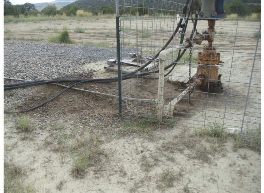
Staining on ground at wellhead
