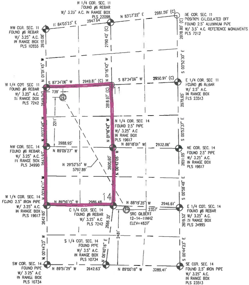
IN ACCORDANCE WITH A REQUEST FROM CRAIG RASMUSON - SYNERGY RESOURCES, BASELINE ENGINEERING CORP HAS DETERMINED THE LOCATION OF THE SRC GILBERT 12-14-11NHZ TO BE 2,481' FSL AND 2,357' FEL, AS MEASURED AT NINETY (90) DEGREES FROM THE SECTION LINE OF SECTION 14, TOWNSHIP 5 NORTH, RANGE 66 WEST AND THE BOTTOM HOLE LOCATION TO BE 2,211' FSL AND 739' FWL OF SECTION 11, TOWNSHIP 5 NORTH, RANGE 66 WEST, 6TH PRINCIPAL MERIDIAN, WELD COUNTY, COLORADO
