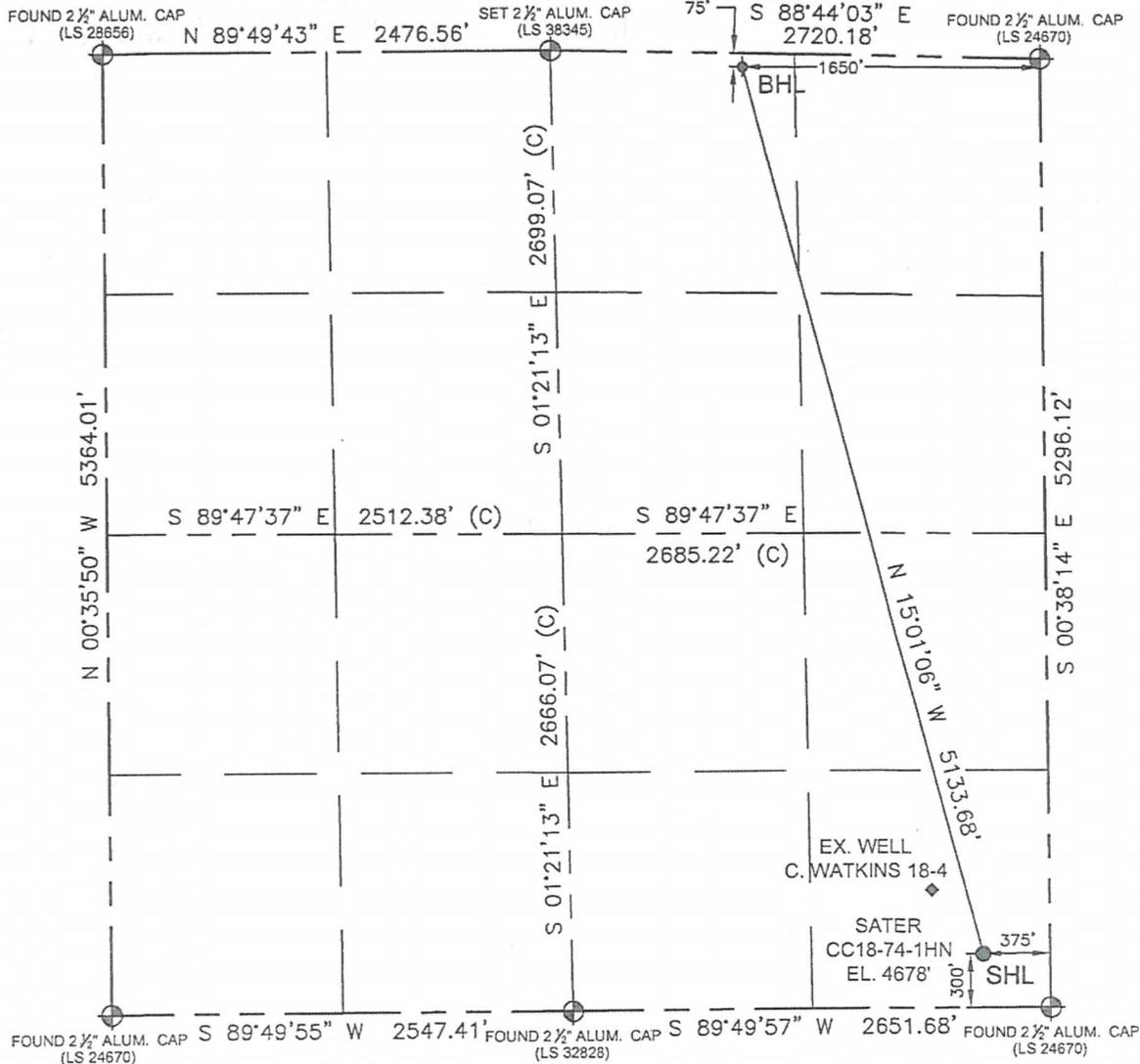
In accordance with a request from Matt Verbit with Noble Energy Inc. Petroleum Field Services, LLC has determined the surface location of the SATER CC18-74-1HN to be 300' from the SOUTH line and 375' from the EAST line and the bottom hole to be 75' from the NORTH line and 1650' from the EAST line as measured at right angles from the section line of Section 18, Township 4 North, Range 63 West of the Sixth Principal Meridian, County of WELD, State of Colorado.
