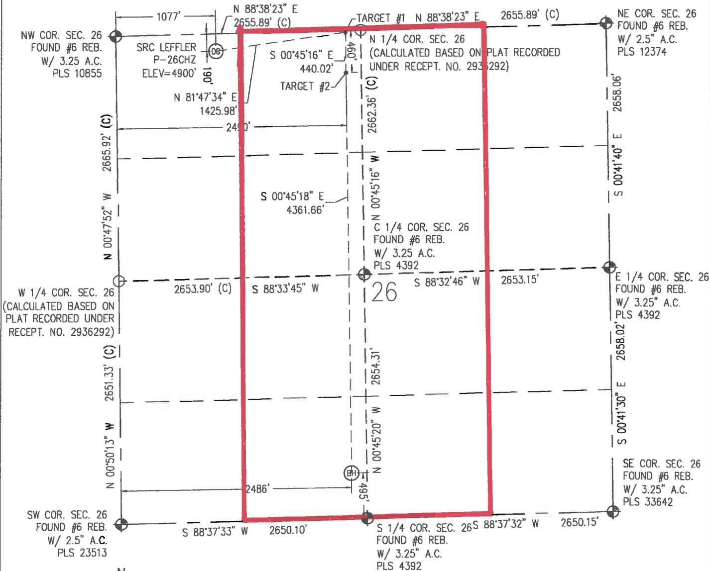
IN ACCORDANCE WITH A REQUEST FROM CRAIG RASMUSON - SYNERGY RESOURCES, BASELINE ENGINEERING CORP. HAS DETERMINED THE LOCATION OF THE SRC LEFFLER P-26CHZ TO BE 190' FNL AND 1077' FWL, AS MEASURED AT NINETY (90) DEGREES FROM THE SECTION LINE OF SECTION 26, TOWNSHIP 7 NORTH, RANGE 66 WEST AND THE BOTTOM HOLE LOCATION TO BE 495' FSL AND 2486' FWL OF SECTION 26, TOWNSHIP 7 NORTH, RANGE 66 WEST, 6TH PRINCIPAL MERIDIAN, WELD COUNTY, COLORADO.
