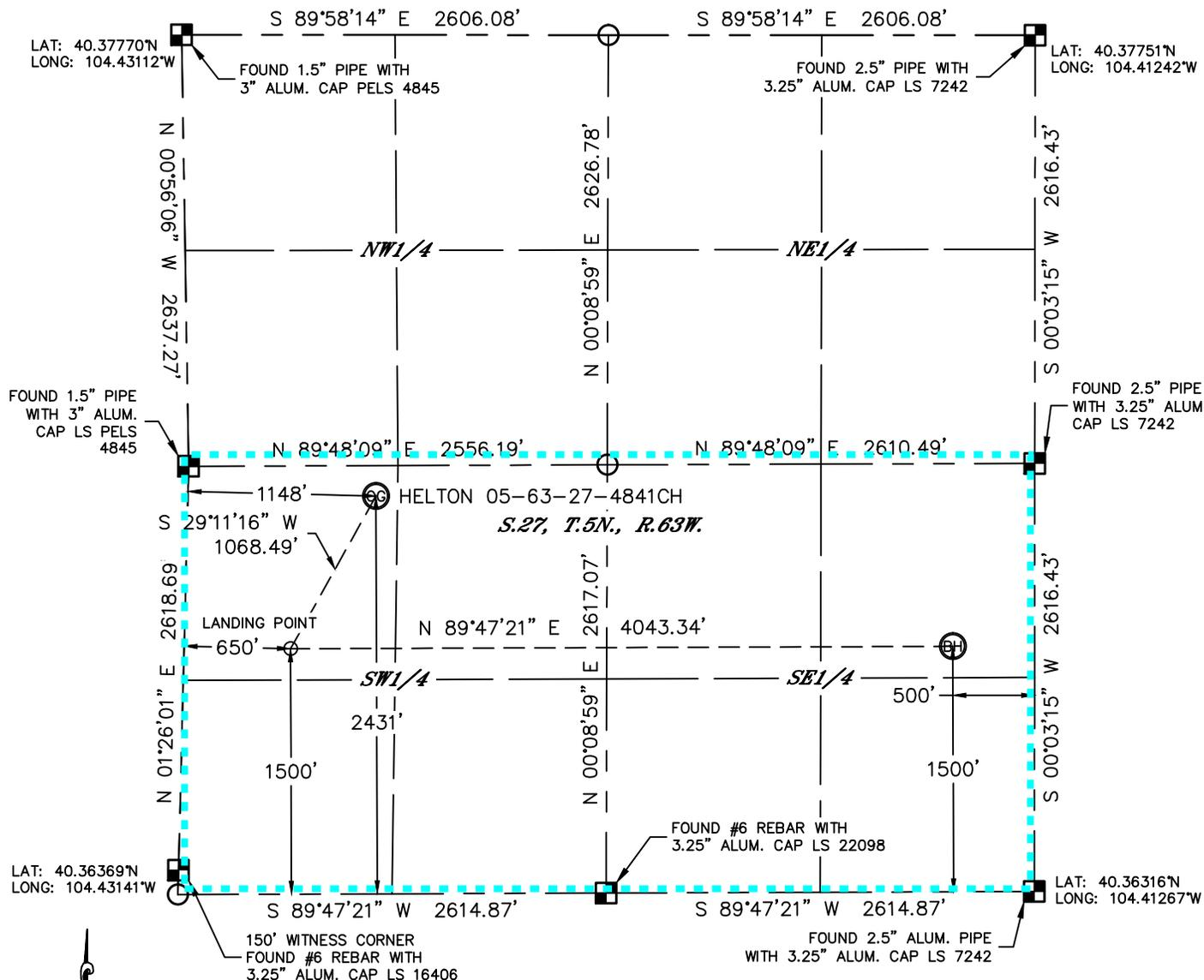
In accordance with a request from Jeff Fandrich with BILL BARRETT CORPORATION Lat40°, Inc. has determined the surface location of the HELTON 05-63-27-4841CH to be 2431' from the SOUTH line and 1148' from the WEST line and the bottom hole to be 1500' from the SOUTH line and 500' from the EAST line as measured at right angles from the section lines of Section 27, Township 5 North, Range 63 West of the Sixth Principal Meridian, County of Weld, State of Colorado.
