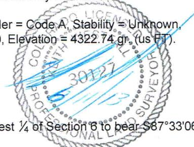
**Basis of Bearing:** Bearings were determined based on the North line of the Northwest 1/4 of Section 6 to bear **S87°33'06"W** with all other bearings contained herein relative thereto.
