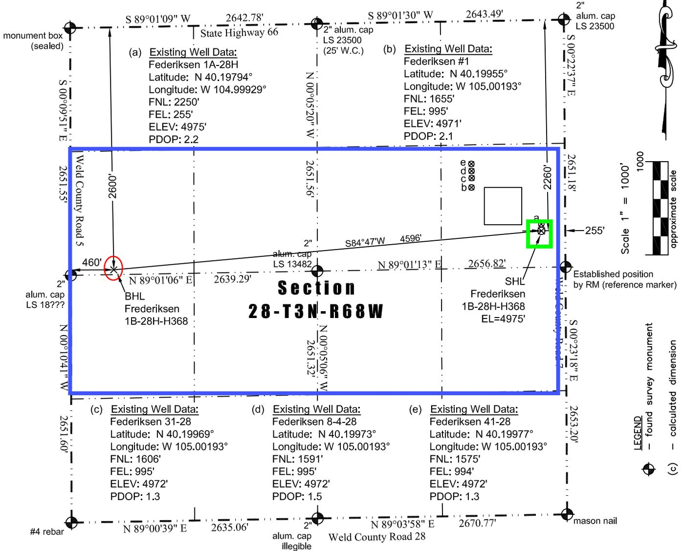
In accordance with a request from Jay Knutson of EnCana Oil & Gas (USA) Inc., JR Land Surveying, LLC has determined the location of the **Frederiksen 1B-28H-H368** well site to be SHL: 2260' FNL and 255' FEL, (BHL: 2600' FNL and 460' FWL), as measured at ninety (90) degrees from the section lines of Section 28, Township 3 North, Range 68 West of the 6th Principal Meridian, Weld County Colorado.
