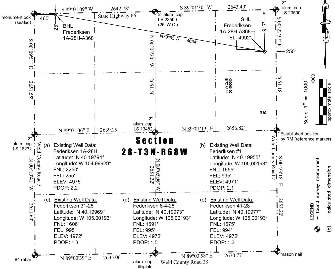
In accordance with a request from Jay Knutson of EnCana Oil & Gas (USA) Inc., JR Land Surveying, LLC has determined the location of the **Federiksen 1A-28H-A368** well site to be SHL: 917' FNL and 250' FEL, (BHL: 25' FNL and 460' FWL), as measured at ninety (90) degrees from the section lines of Section 28, Township 3 North, Range 68 West of the 6th Principal Meridian, Weld County Colorado.
