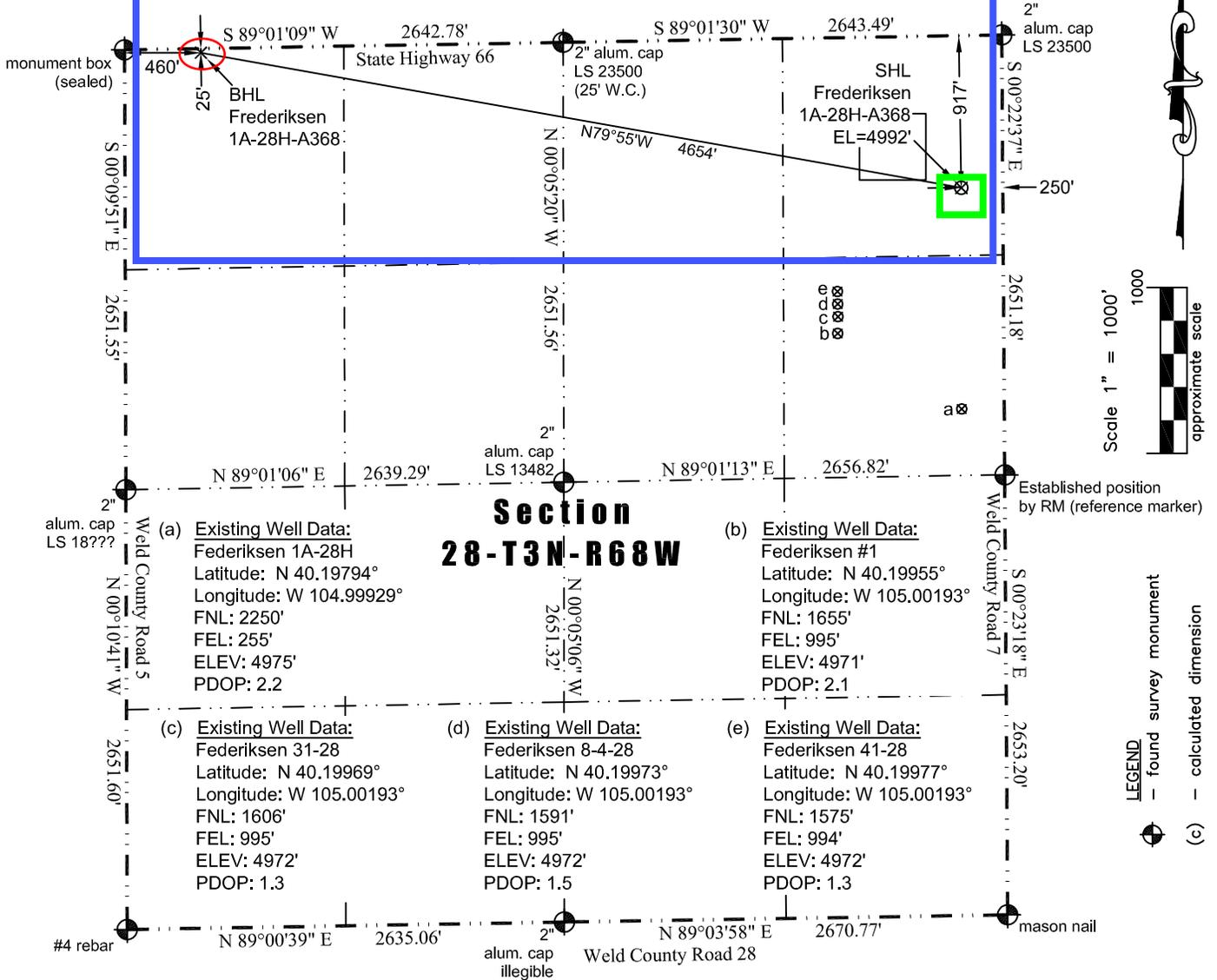
In accordance with a request from Jay Knutson of EnCana Oil & Gas (USA) Inc., JR Land Surveying, LLC has determined the location of the **Frederiksen 1A-28H-A368** well site to be SHL: 917' FNL and 250' FEL, (BHL: 25' FNL and 460' FWL), as measured at ninety (90) degrees from the section lines of Section 28, Township 3 North, Range 68 West of the 6th Principal Meridian, Weld County Colorado.
