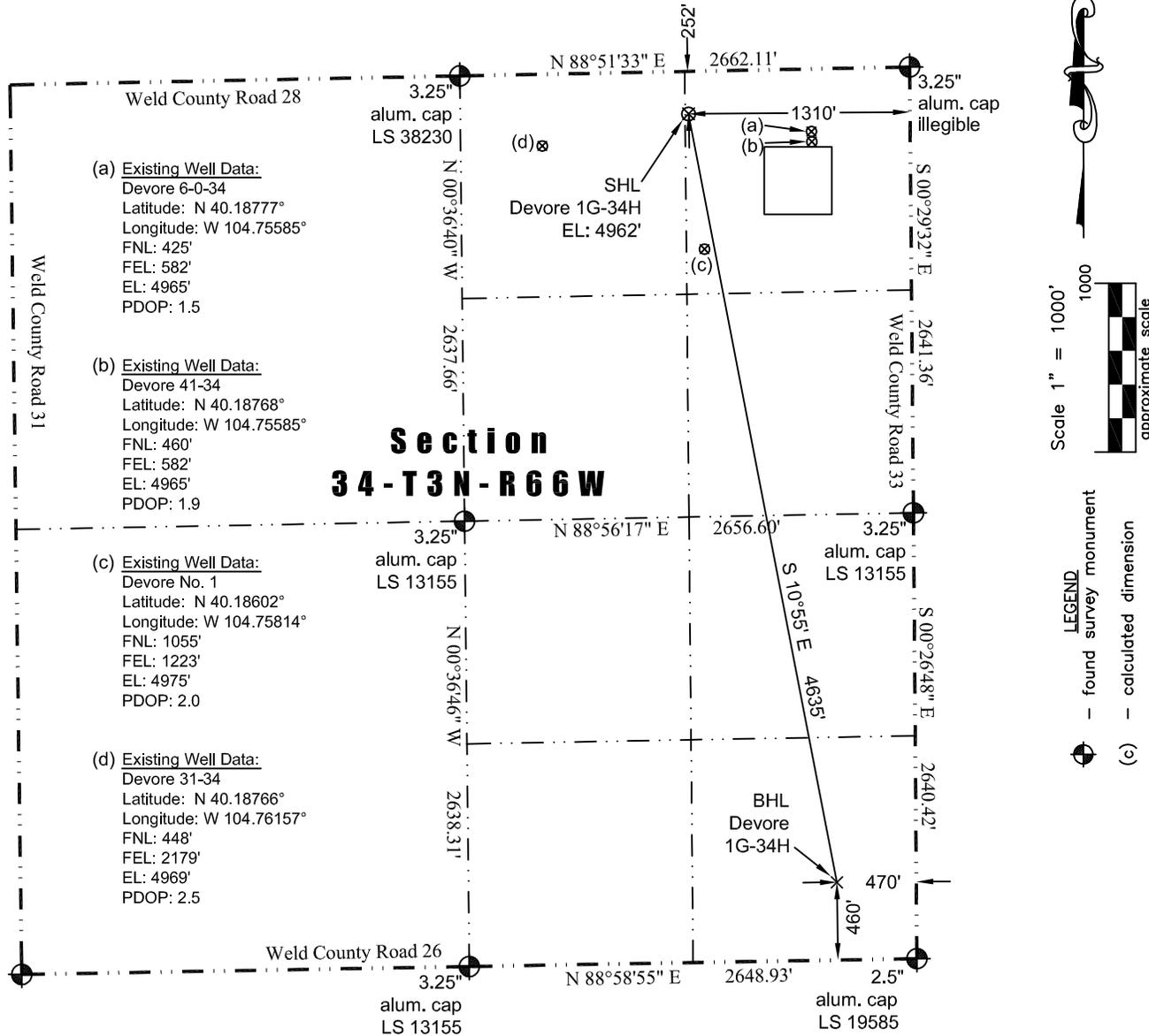
In accordance with a request from Jay Knutson of EnCana Oil & Gas (USA) Inc., JR Land Surveying, LLC has determined the location of the **Devore 1G-34H** well site to be SHL: 252' FNL and 1310' FEL, (BHL: 460' FSL and 470' FEL), as measured at ninety (90) degrees from the section lines of Section 34, Township 3 North, Range 66 West, 6th Principal Meridian, Weld County, CO.
