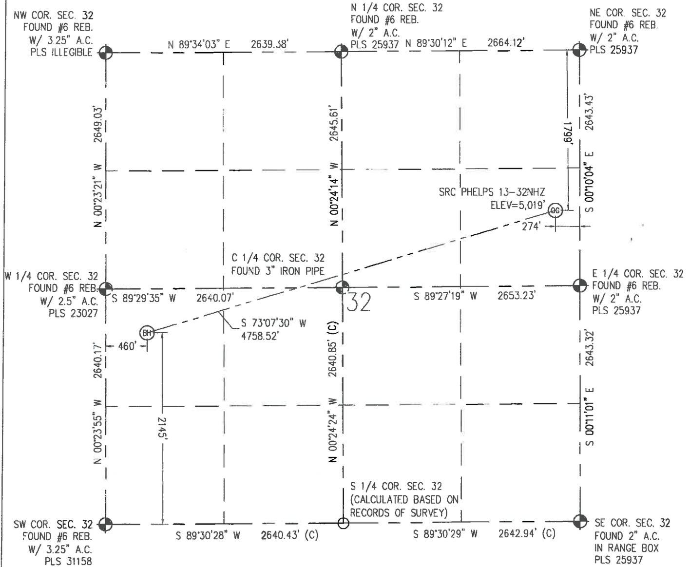
IN ACCORDANCE WITH A REQUEST FROM CRAIG RASMUSON - SYNERGY RESOURCES, BASELINE ENGINEERING CORP. HAS DETERMINED THE LOCATION OF THE SRC PHELPS 13-32NHZ TO BE 1,799' FNL AND 274' FEL, AS MEASURED AT NINETY (90) DEGREES FROM THE SECTION LINE OF SECTION 32, TOWNSHIP 1 NORTH, RANGE 66 WEST AND THE BOTTOM HOLE LOCATION TO BE 2,145' FSL AND 460' FWL OF SECTION 32, TOWNSHIP 1 NORTH, RANGE 66 WEST, 6TH PRINCIPAL MERIDIAN, WELD COUNTY, COLORADO
