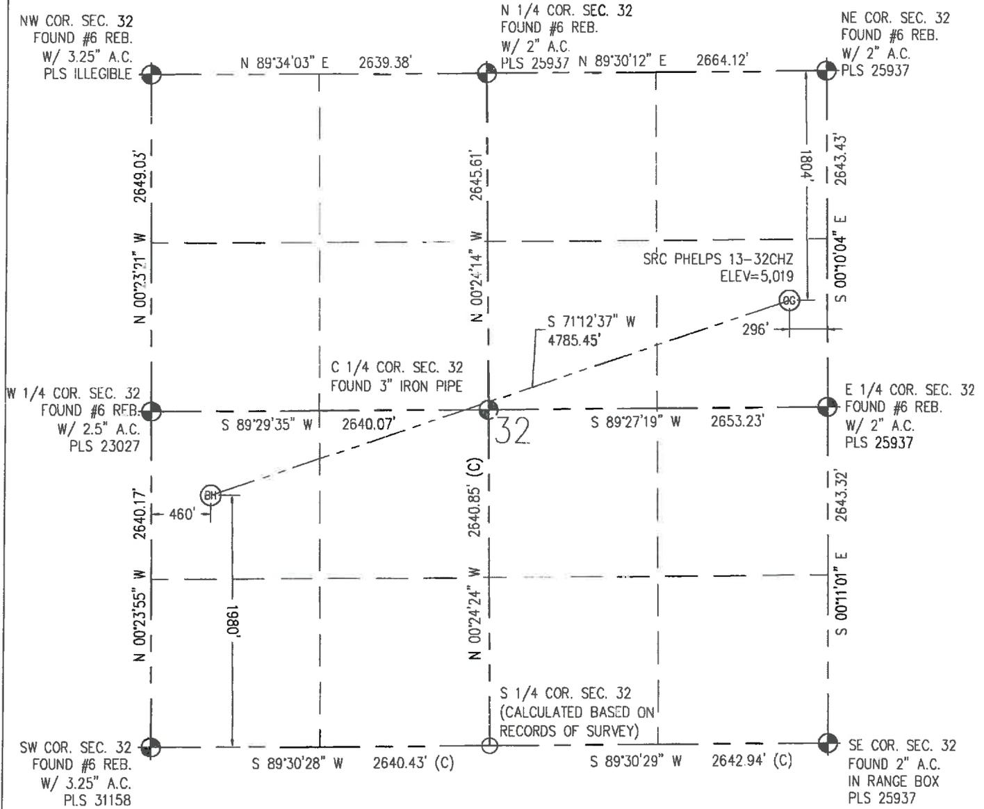
IN ACCORDANCE WITH A REQUEST FROM CRAIG RASMUSON - SYNERGY RESOURCES, BASELINE ENGINEERING CORP. HAS DETERMINED THE LOCATION OF THE SRC PHELPS 13-32CHZ TO BE 1,804' FNL AND 296' FEL, AS MEASURED AT NINETY (90) DEGREES FROM THE SECTION LINE OF SECTION 32, TOWNSHIP 1 NORTH, RANGE 66 WEST AND THE BOTTOM HOLE LOCATION TO BE 1,980' FSL AND 460' FWL OF SECTION 32, TOWNSHIP 1 NORTH, RANGE 66 WEST, 6TH PRINCIPAL MERIDIAN, WELD COUNTY, COLORADO.
